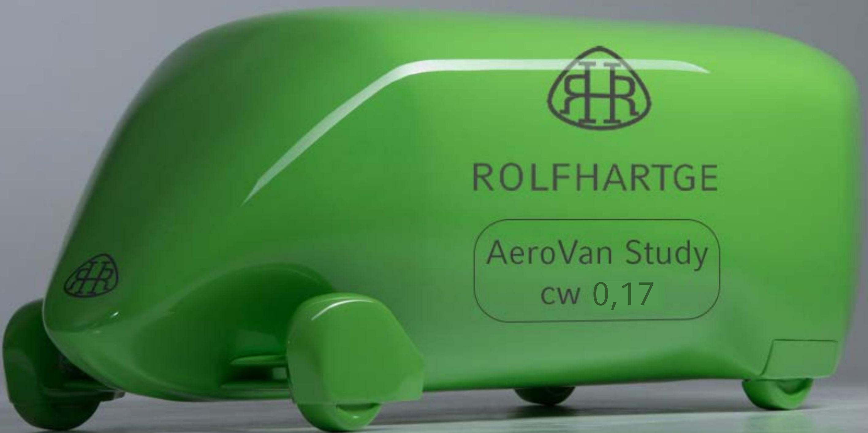
The wind tunnel measurements of the AeroVan 1:5 model have revealed the best value of  $c_w = 0.20$ . This result corresponds to the value of the current aerodynamics world champion Mercedes-Benz EQS – energy instead of fuel consumption.
